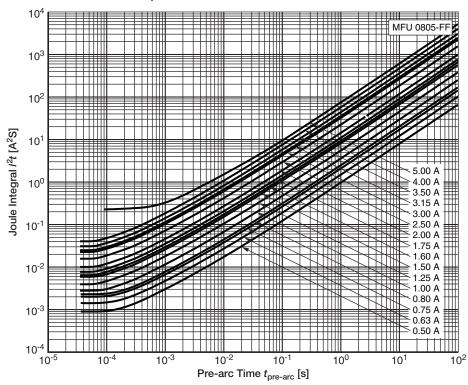
Typical  $\mathit{I}^{2}t$  vs.  $t_{\mathrm{pre-arc}}$  characteristic of MFU 0805 <sup>(1)</sup>
