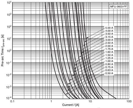
Typical  $t_{\mathrm{pre-arc}}$  vs. I characteristic of MFU 0603  $^{(1)}$
