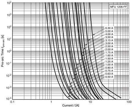
Typical  $t_{\rm pre-arc}$  vs. I characteristic of MFU 1206 <sup>(1)</sup>
