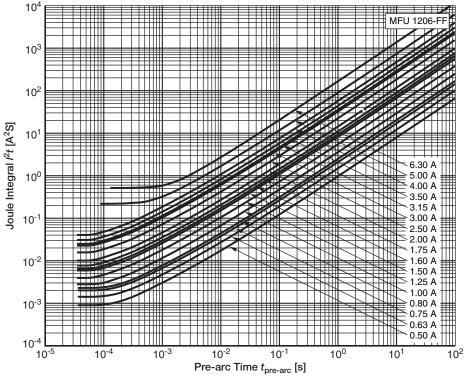
Typical  $I^2t$  vs.  $t_{pre-arc}$  characteristic of MFU 1206 (1)
