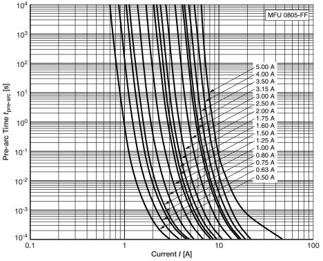
Typical  $t_{\rm pre-arc}$  vs. I characteristic of MFU 0805  $^{(1)}$
