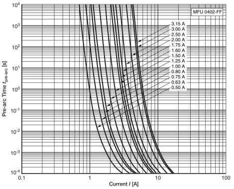
Typical  $t_{\rm pre-arc}$  vs. I characteristic of MFU 0402 <sup>(1)</sup>
