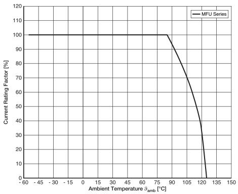
Current Rating Factor (1) vs. Ambient Temperature  $\vartheta_{amb}$
