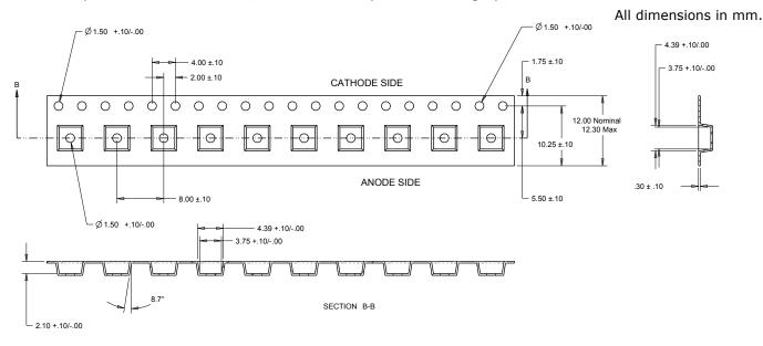
Notes: 1. 10 sprocket hole pitch cumulative tolerance ± 0.2mm
