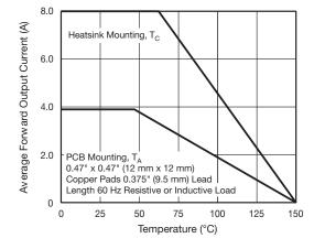
Fig. 1 - Derating Curve Output Rectified Current
