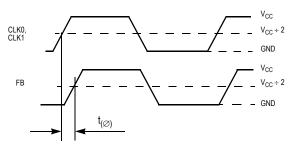
Figure 13. Propagation Delay  $(\mathbf{t}_{(\emptyset)},$  static phase offset) Test Reference
