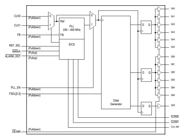
Figure 1. MPC9893 Logic Diagram
