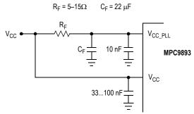
Figure 3. V<sub>CC PLL</sub> Power Supply Filter
