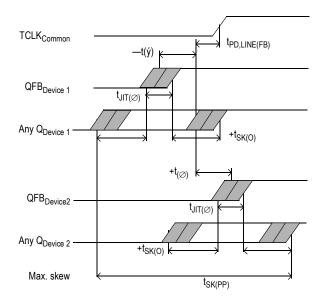
Figure 4. MPC9893 Max. Device-to-Device Skew
