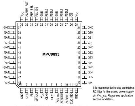
Figure 2. MPC9893 48-Lead Pinout (Top View)
