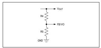
Figure 1. Setting the Output Voltage
