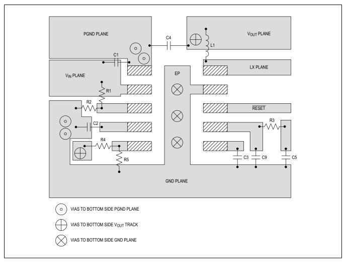
Figure 5. Recommended Component Placement for MAX17501G/H
