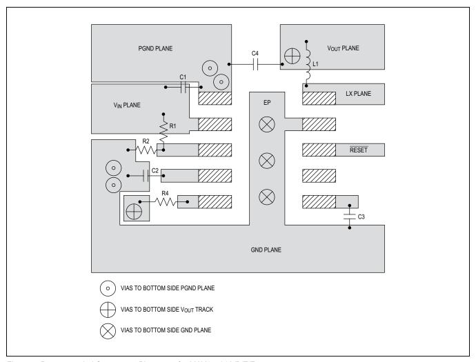
Figure 4. Recommended Component Placement for MAX17501A/B/E/F
