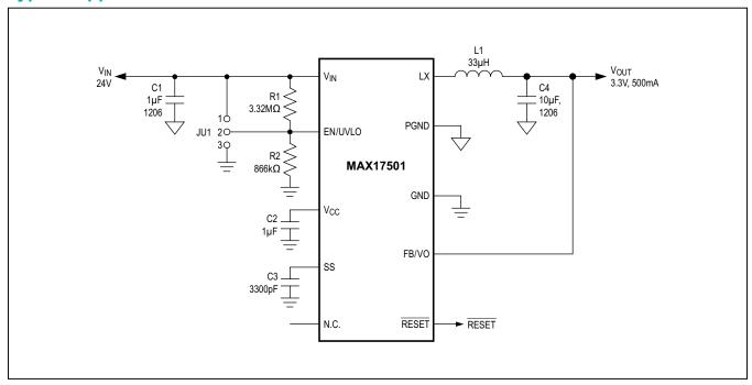
Figure 6. MAX17501A/E Application Circuit (3.3V Output, 500mA Maximum Load Current, 600kHz Switching Frequency)
