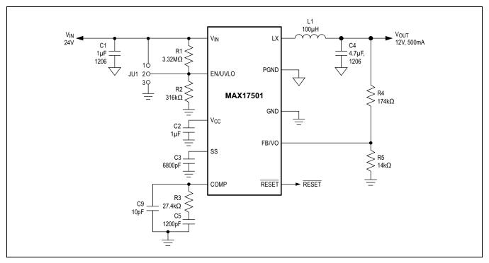
Figure 8. MAX17501G Application Circuit (12V Output, 500mA Maximum Load Current, 600kHz Switching Frequency)
