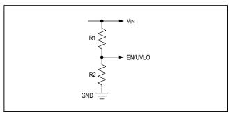
Figure 2. Adjustable EN/UVLO Network
