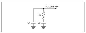
Figure 3. External Compensation Network
