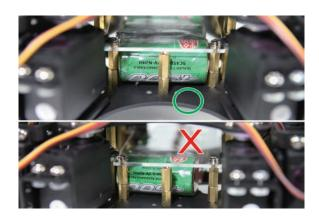
5. Check if the battery is installed properly from the other side. The battery needs to be center placed.
