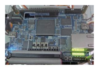
The Spider will begin to stand up after LED7 blinks for 10 seconds. LED0~6 will stay on once the initialization is completed.
