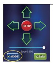
14. Press the "K-Mode" button will switch to "G-sensor" mode. Switch again will return to the default mode controlled by The four Arrow Buttons.
