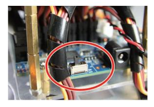
7. Switch the Power Switch on the Servo Motor Card to "ON" position.
