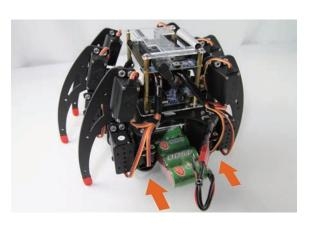
4. Install the battery into the Spider Robot from behind.
