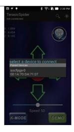
12. If the connection is established successfully, the color of Bluetooth logo will turn to green. The Spider can now be controlled from the cell phone.
