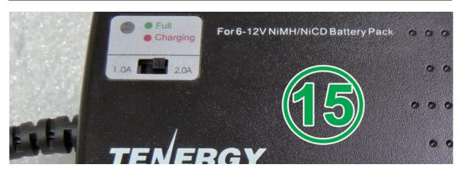
1. Switch the current of "(15)Battery Charger" to 2.0A.
