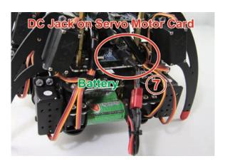
6. Connect the battery to the DC Jack on the Servo Motor Card via " Battery to DC Jack Cable".
