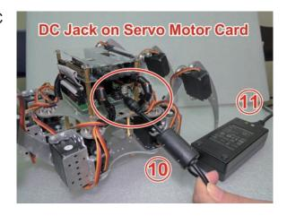
4. Switch the Power Switch on the Servo Motor Card to "ON" position.
