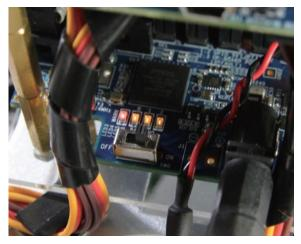
There is a CPLD on the Servo Motor Card to manage the power supplied to the Servo Motors. It provides battery level indication and is responsible for powering off the spider when the battery low or power consumption is too large. There are three orange LEDs and one red LED on the Servo Motor Card for the indication of power status. The three orange LEDs indicate the power level of the battery. The red LED indicates the status of power exception.
