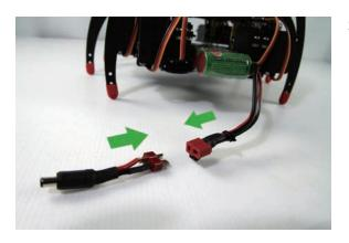
3. Connect the Batter-to-DC jack cable to the battery.
