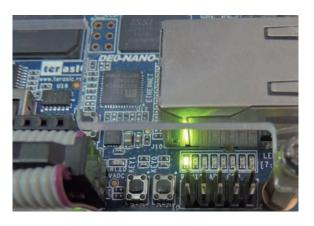
6. The Spider will begin to stand up after LED7 blinks for 10 seconds. LED0~6 will stay on once the initialization is completed.
