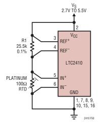
Figure 50. Remote Half Bridge Interface
