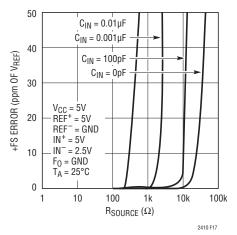
Figure 17. +FS Error vs  $R_{SOURCE}$  at IN<sup>+</sup> or IN<sup>-</sup> (Small C<sub>IN</sub>)
