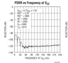
PSRR vs Frequency at  $V_{\mbox{CC}}$
