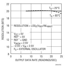
Figure 31. Resolution (INL<sub>RMS</sub>  $\leq$  1LSB) vs Output Data Rate and Temperature
