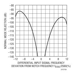
Figure 4. LTC2410 Normal Mode Rejection When Using an External Oscillator of Frequency f<sub>EOSC</sub>
