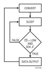
Figure 2. LTC2410 State Transition Diagram
