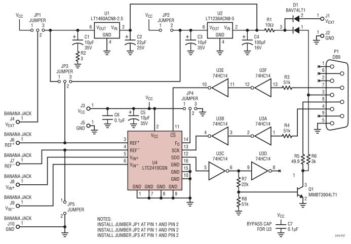
Figure 57. 24-Bit A/D Demo Board Schematic
