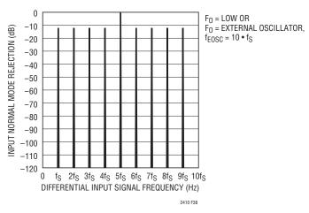
Figure 38. Input Normal Mode Rejection, Internal Oscillator and 60Hz Notch or External Oscillator
