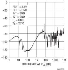
PSRR vs Frequency at V<sub>CC</sub>
