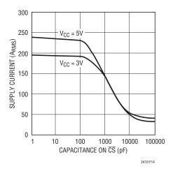
Figure 14.  $\overline{\text{CS}}$  Capacitance vs Supply Current
