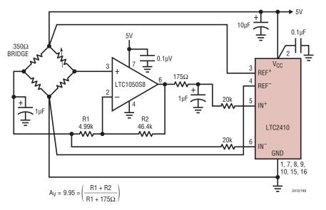
Figure 49. Bridge Amplification Using a Single Amplifier
