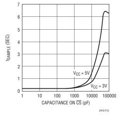
Figure 12.  $\overline{\text{CS}}$  Capacitance vs  $t_{\text{SAMPLE}}$
