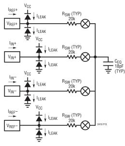
$\begin{array}{l} \mbox{SWITCHING FREQUENCY} \\ f_{SW} = 76800 \mbox{Hz INTERNAL OSCILLATOR (F_0 = LOW OR HIGH)} \\ f_{SW} = 0.5 \bullet f_{EOSC} \mbox{EXTERNAL OSCILLATOR} \end{array}$
