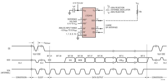
Figure 8. Internal Serial Clock, Single Cycle Operation
