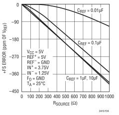
Figure 24. +FS Error vs  $R_{SOURCE}$  at REF<sup>+</sup> or REF<sup>-</sup> (Large  $C_{REF}$ )
