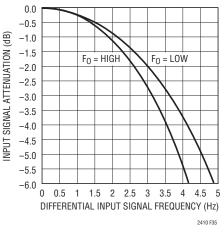
Figure 35. Input Signal Bandwidth Using the Internal Oscillator
