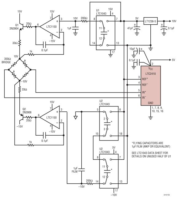
Figure 52. LTC1043 Provides Precise 4× Reference for Excitation Voltages
