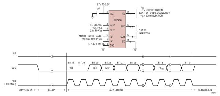
Figure 7. External Serial Clock,  $\overline{CS} = 0$  Operation (2-Wire)
