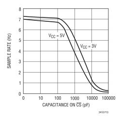
Figure 13.  $\overline{\text{CS}}$  Capacitance vs Output Rate
