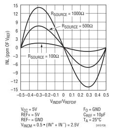
Figure 26. INL vs Differential Input Voltage ( $V_{IN} = IN^+ = IN^-$ ) and Reference Source Resistance ( $R_{SOURCE}$  at REF<sup>+</sup> and REF<sup>-</sup>) for Large  $C_{REF}$  Values ( $C_{REF} \ge 1\mu F$ )
