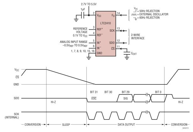
Figure 11. Internal Serial Clock, Autostart Operation
