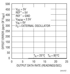
Figure 27. Offset Error vs Output Data Rate and Temperature
