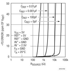
Figure 23. –FS Error vs  $R_{SOURCE}$  at REF<sup>+</sup> or REF<sup>-</sup> (Small C<sub>IN</sub>)
