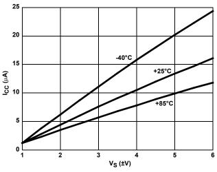
FIGURE 17. SUPPLY CURRENT vs SUPPLY VOLTAGE
