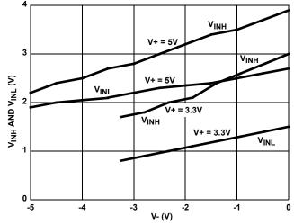
FIGURE 14. DIGITAL SWITCHING POINT vs NEGATIVE SUPPLY VOLTAGE
