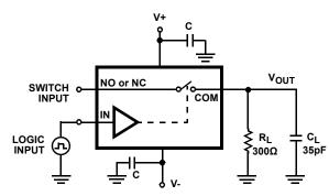
C<sub>L</sub> includes fixture and stray capacitance.
