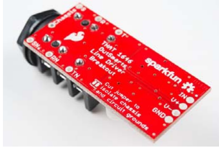
Closeup of ground jumper.
