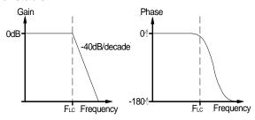
Fig. 13: Gain and Phase of LC filter
