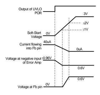
Fig. 6: Theoretical operation waveforms during soft-start
