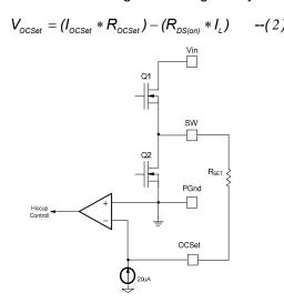
Fig. 7: Connection of over current sensing resistor
