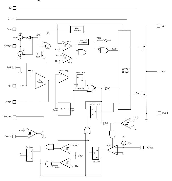
Fig. 3. Simplified block diagram of the IR3822A.
