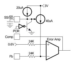
Fig. 5: Soft-Start circuit for IR3822A
