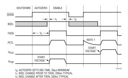
NOTE 1: THE EXTERNAL DAC DRIVING THE PCTL PIN CAN BE ENABLED DURING AUTOZERO. THE AUTOZERO SYSTEM WILL CANCEL THE DAC TRANSIENT. THE DAC MUST BE SETTLED TO AN OFFSET ≤400mV BEFORE TXEN IS ASSERTED HIGH.
