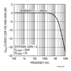
Figure 7. SPICE Model Closed Loop Voltage Gain
