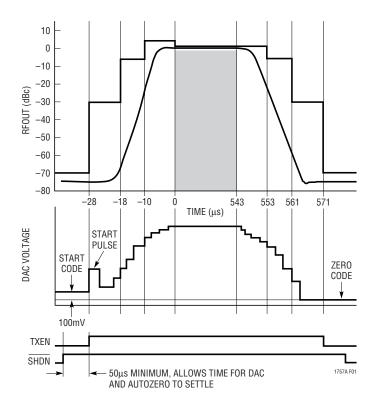
Figure 1. LTC1757A Ramp Timing
