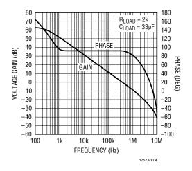
Figure 4. Measured Open Loop Gain and Phase
