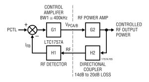
Figure 5. Closed Loop Block Diagram
