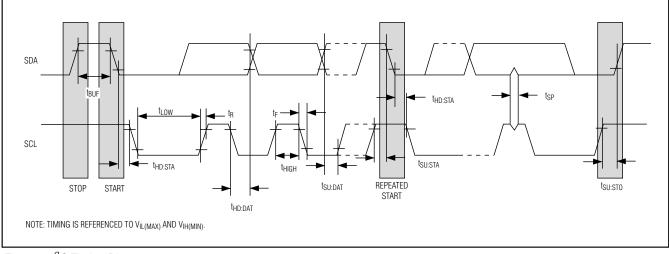
Figure 4. I<sup>2</sup>C Timing Diagram
